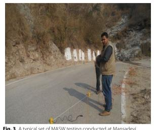
Fig. 3  $\,$  A typical set of MASW testing conducted at Mansadevi landslide
