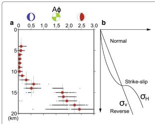
**Fig. 7 a** Relative magnitude of the three principal stress axes,  $A_{\phi}$  plotted against depth in the south part of the forearc.  $A_{\phi}$  was estimated from the focal mechanisms within 2 km of each depth. *Red circles* the best-fit solutions. *Black dots* the 95 % confidence limits (after Yoshida et al. 2015b). **b** Schematic image of the depth variations in the stress field
