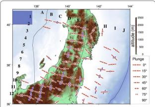
**Fig. 2** Orientations of the best fit  $\sigma_1$  and  $\sigma_3$  axes projected onto a gridded horizontal plane are indicated by *red* and *blue arrows*, respectively. The length of *arrows* varies in proportion to the steepness of the plunge (after Yoshida et al. 2015b)
