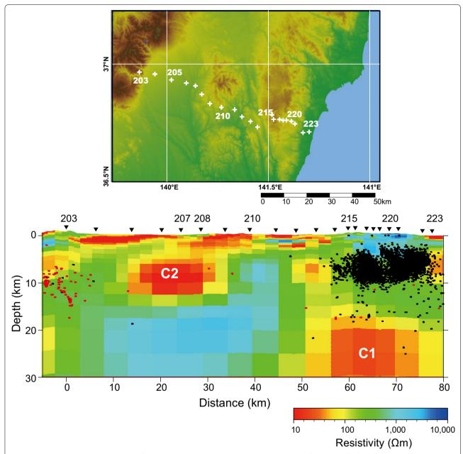
**Fig. 4** 2-D resistivity model. Hypocenters of earthquake swarms (*black dots*) within a 10 km width of the MT profile from March, 2011 to August, 2012, are shown on this figure. Also shown is the hypocenter distribution (*red dots*) before the Tohoku-Oki earthquake, from January 2008 to March 2011, identified by the JMA (after Umeda et al. 2015). *Inset map* the locations of MT stations (*filled crosses*)
