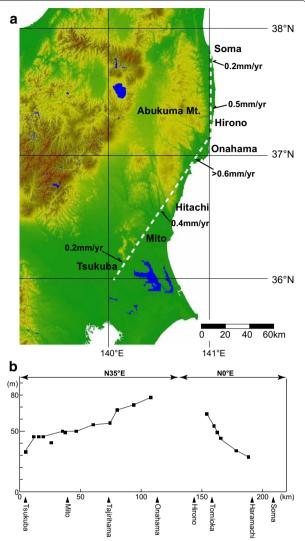
**Fig. 6 a** Late Quaternary uplift rate inferred from marine terraces in the Southeast Tohoku district. **b** Elevations of marine terraces formed during the late Pleistocene along the Pacific coast (*white broken line*), shown in **a** (after Suzuki 1989)
