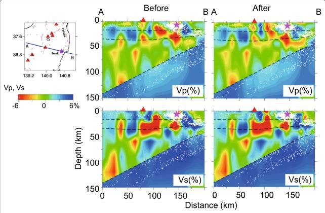
**Fig. 3** Vertical cross-sections of P-wave and S-wave velocity images along the profile as shown in the *inset map* using the data sets from earthquakes that occurred before (*left*) and after (*right*) the 11 March 2011 Tohoku-Oki earthquake (after Zhao 2015)
