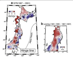
**Fig. 5** Vertical velocities **a** observed by GPS and **b** observed by the recent GSI leveling survey. Contour interval is 5 mm/year. *Blue* and *red areas* denote subsidence and uplift, respectively (after Suwa et al. 2006)
