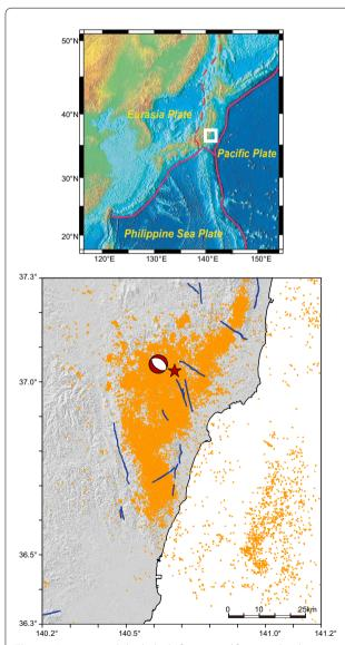
**Fig. 1 a** Location and shaded relief maps, and **b** generalized structure of the Southeast Tohoku district. *Yellow dots* the epicenters of earthquakes identified by the JMA that occurred from March, 2011 to August, 2012 at depths shallower than 20 km. *Red star* and *focal mechanism symbols* (F-net catalog from NIED) indicate the  $M_{\rm w}$  6.7 lwaki earthquake, on April 11. Active faults are also shown (*dark blue lines*) (after Nakata and Imaizumi 2002)
