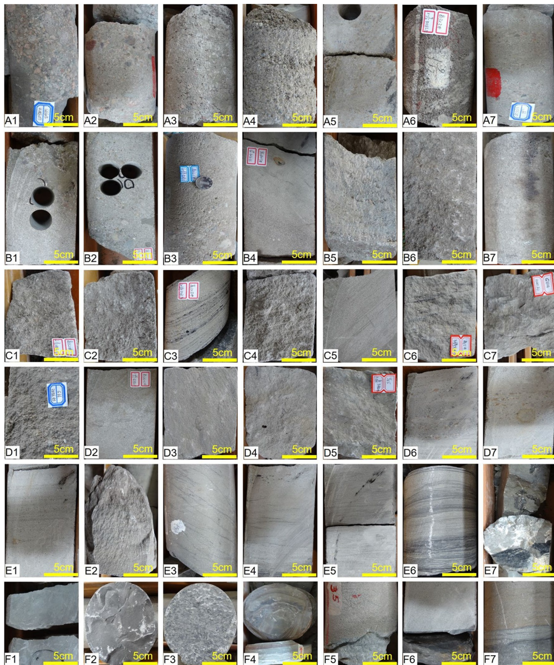
Fig. 7 Typical sedimentary structures of the Shahejie Formation in Nanpu Sag, Bohai Bay Basin. A1: Normal graded cross-bedding, G66×5, A2: Through cross-bedding, G66×5, A3: Through cross-bedding, G3×3, A4: Through cross-bedding, G5, A5: Through cross-bedding, G123×9, A6: Through cross-bedding, oil trace, G3×3, A7: Through cross-bedding, G66, B1: Inverse graded cross-bedding, G66×5, B2: Normal graded cross-bedding, very coarse-grained, G66-3, B3: Normal graded cross-bedding, G66-1, B4: Normal graded cross-bedding, G66-3, B5: Through cross-bedding, G19-10, B6: Through cross-bedding, oil trace, G19-10, B7: Through cross-bedding, G82, C1: Low angle cross-bedding, G82, C2: High angle cross-bedding, G83-10, C3: High angle cross-bedding, G3×3, C4: Low angle cross-bedding, G19-10, C5: High angle cross-bedding, G66×5, C6: Through cross-bedding, G5, C7: Through cross-bedding, G3104, D1: Normal graded cross-bedding, G66, D2: Massive bedding, G66×5, D3: Massive bedding, fault plane, G5, D4: Massive bedding, oil trace, G5, D5: Massive bedding, G5, D6: Parallel bedding, G123×9, D7: Parallel bedding, G123×9, E1: Parallel bedding, G123×9, E2: Parallel bedding, G32-30, E3: Ripple cross-bedding, G3×3, E4: Inverse graded, Ripple cross-bedding, G123×9, E5: Ripple cross-bedding, G123×9, E6: Composite bedding, G8×1, E7: Fault plane, Asphaltene, G66×5, F1: Mud, G66×3, F2: Mud, Inverse graded, F3: Mud, G65-1, F4: Mud, G3104, F5: Erosion surface, G5, F6: Erosion surface, G83-10, F7: Erosion surface, G8×1
