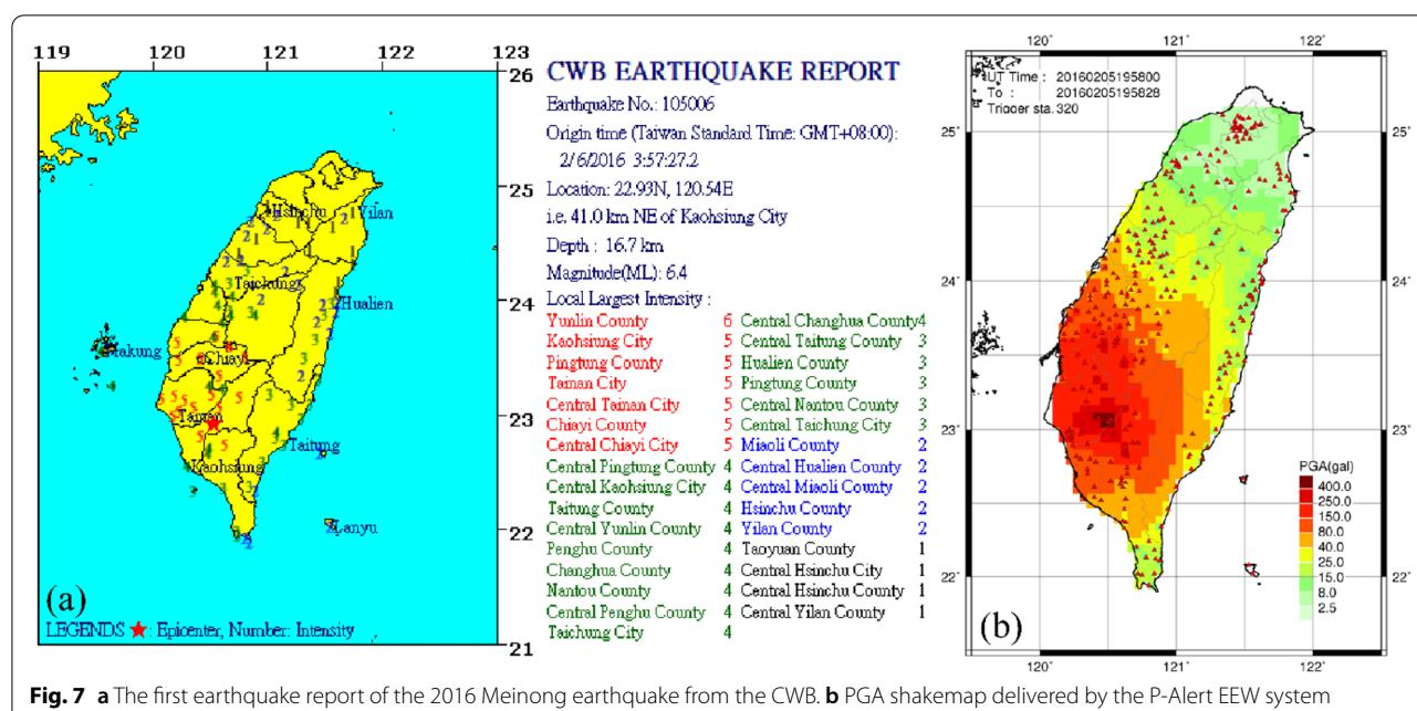
**Fig. 7** **a** The first earthquake report of the 2016 Meinong earthquake from the CWB. **b** PGA shakemap delivered by the P-Alert EEW system
