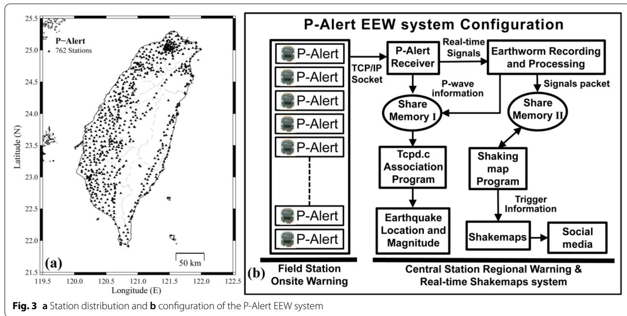
**Fig. 3** **a** Station distribution and **b** configuration of the P-Alert EEW system
