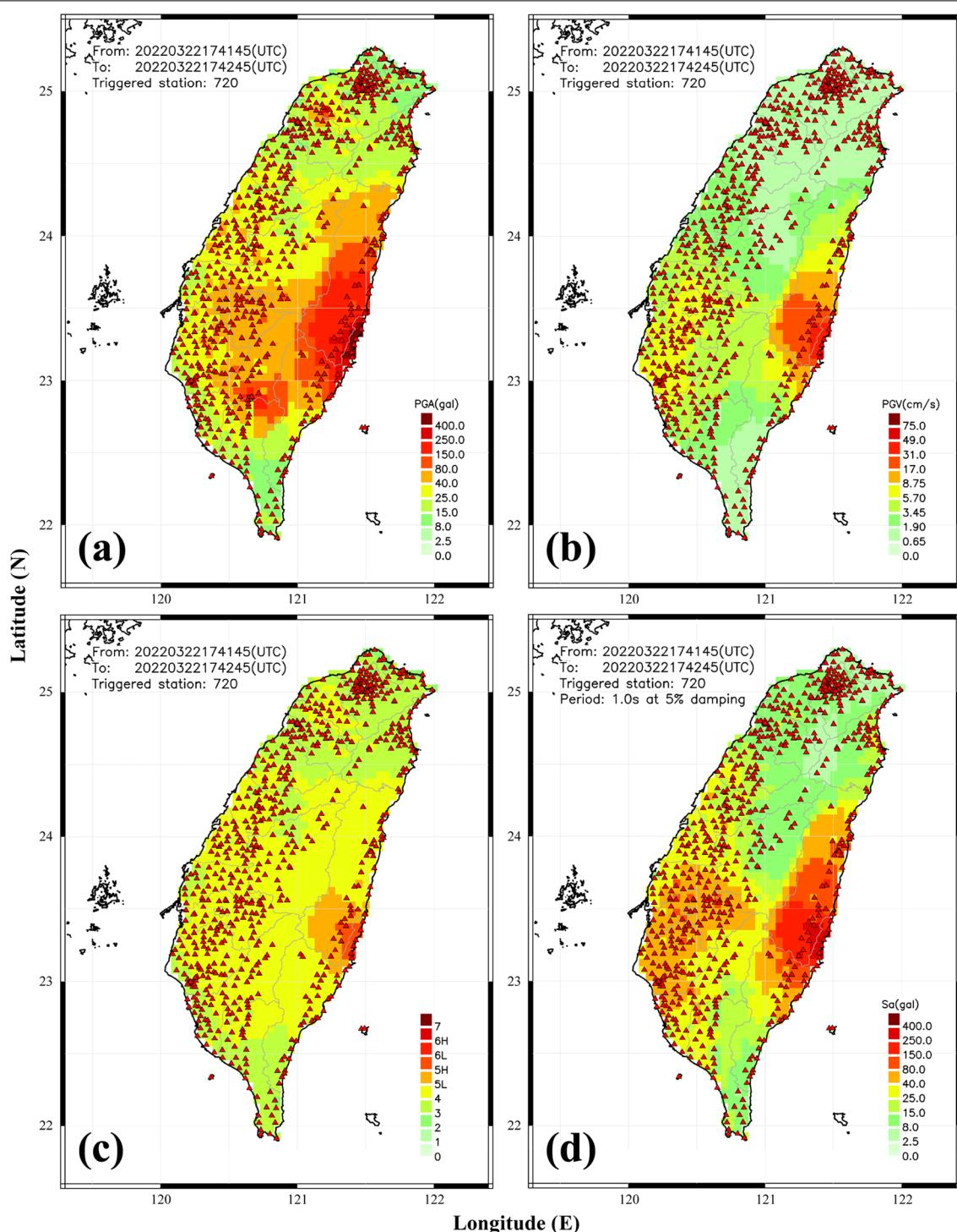
**Fig. 5** **a** PGA, **b** PGV, **c** CWB intensity, and **d** 1 s  $S_a$  shakemaps delivered from the P-Alert EEW system for March 22, 2022,  $M_w$  6.6 eastern Taiwan earthquake
