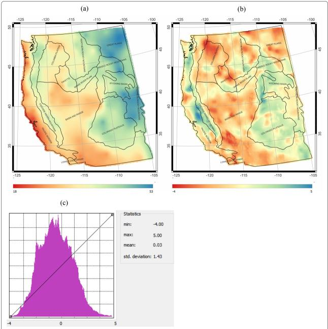
Fig. 12 a Moho depth (km) from CRUST 1.0 model, b calculated misfit map (km) between our estimates of Moho and CRUST 1.0 model in the study area, c misfit between the estimated Moho depths from gravity inversion and Moho depths from the CRUST 1.0 model
