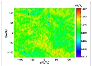
**Figure 1** Time snapshot of elongated structures containing both filaments and propagating waves in the direction to the mean magnetic field direction (in the *z*-direction) for the large-box setting.
