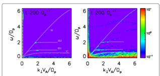
Figure 2 Magnetic energy spectrum  $E\left(k_{\perp},\omega\right)$  averaged over the spatial coordinates parallel to the large-scale magnetic field for two simulation boxes at an earlier evolution time (200 ion gyroperiods,  $t\Omega_{\rm p}=$  200). The wave modes are marked by IB1 (ion Bernstein  $\omega/\Omega_{p}=$  1), IB2 (ion Bernstein  $\omega/\Omega_{p}=$  2), IC (ion cyclotron), and W (whistlers).
