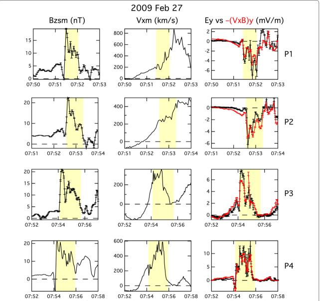
**Fig. 1** The  $B_z$  component, plasma bulk flow, and comparison between  $E_y$  and  $-(V \times B)_y$  for four THEMIS satellites on 2009 February 27. The parameters  $E_y$  and  $-(V \times B)_y$  are in dsl (close to GSE) coordinates
